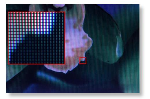
Each pixel consists of three tiny bars (LEDs), each of which emits red, green, or blue in different intensities. Our eye or brain blends them into one of the millions of possible colors.
